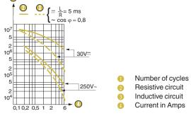
The operating curve relates to contact life, but switch durability is also limited by mechanical life of operating device : see "Mechanical life"
